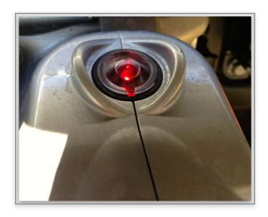
The red light on the CHAdeMO connector plugged in to your LEAF turns **RED**. **This is very important** - and has tripped up many a dear soul. **If it is not red you are not charging!** No red light means that the CHAdeMO connector is not seated properly. Go back and very carefully pull up on the lever while simultaneously pushing the CHAdeMO plug in to the LEAF connector. <sup>3</sup>
